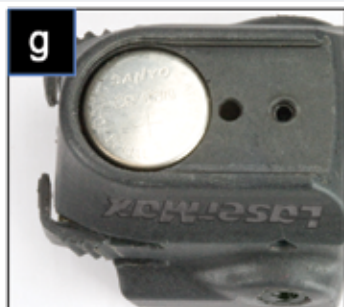
The negative side of the battery goes into the chamber first. The correct orientation of the batteries shown above.
