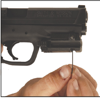
The hole at the bottom adjusts elevation (vertical alignment).
