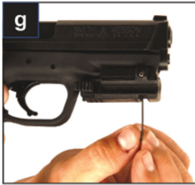
The hole at the bottom adjusts elevation (vertical alignment). A clockwise turn (left side, to front, to right side of firearm) shifts laser down.
