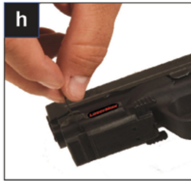
The hole at the side adjusts windage (horizontal alignment). A clockwise turn (front, to top, to bottom) shifts laser to the left.
