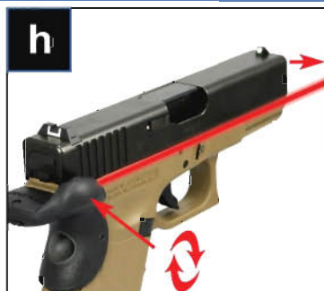
The hole at the side adjusts windage (horizontal alignment). A clockwise turn shifts laser to the right.
