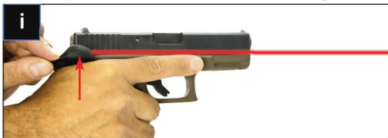
The hole at the top adjusts elevation (vertical alignment). A clockwise turn shifts laser up.
