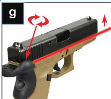
The hole at the top adjusts elevation (vertical alignment). A clockwise turn shifts laser up.
